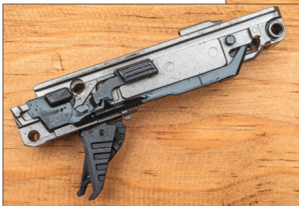
(Above) The Masada Slim disassembles quickly and offers good access for a thorough cleaning. (Left) The modular trigger chassis is the serialized "firearm" component that can be swapped from frame to frame.
