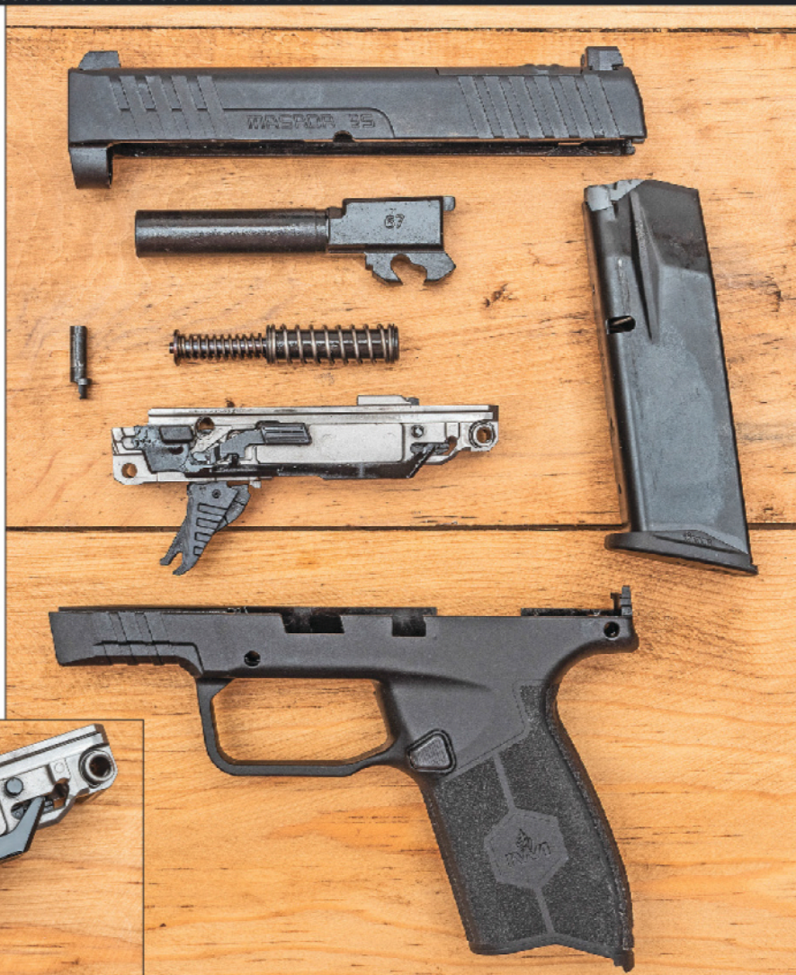
(Above) The Masada Slim disassembles quickly and offers good access for a thorough cleaning. (Left) The modular trigger chassis is the serialized "firearm" component that can be swapped from frame to frame.
